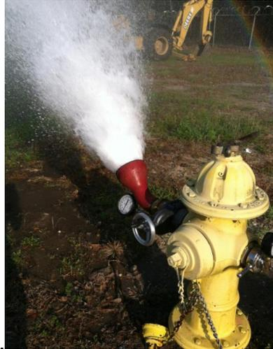
13. Once the hydrant test valve is fully open and the pressure has settled, record the residual pressure on the static gauge and then pitot pressure on the pitot gauge. The residual pressure records both the domestic demand and fire flows occurring in the water main. The pitot is measuring the velocity pressure of the stream discharging from the flow hydrant.
