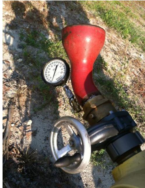
7. Confirm the direction of operation on the hydrant.
