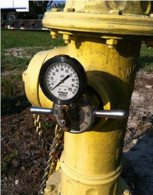
Hydrant Test Valve Diffuser/Pitot
